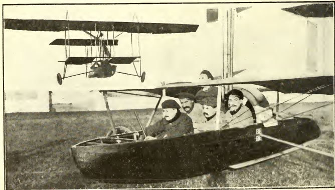
A Henry Farman experimental hydro-biplane (80-h.p. Gnome engine) of new design.—Above the machine is shown flying.
